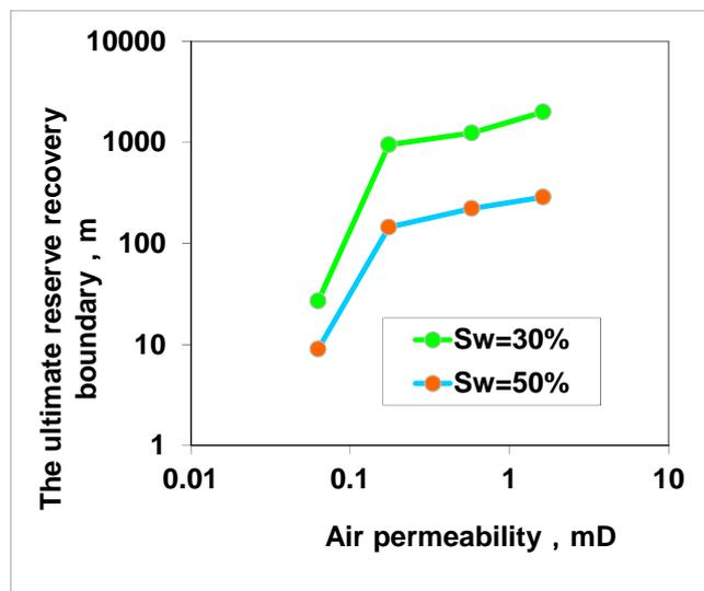
**Fig. 3** The Relation of Ultimate Reserve Recovery Radius and Permeability, Water Saturation at a Pressure of 30 MPa
