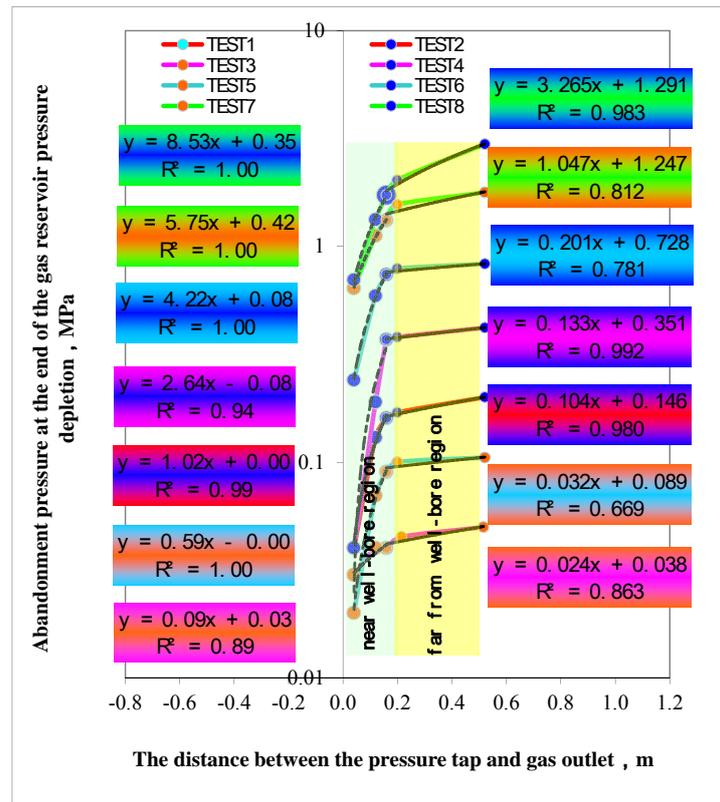
Fig. 2 The Abandonment Formation Pressure Distribution Characteristics
