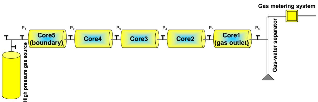
**Fig. 1** The Experiment Workflow and the Location of Pressure Tap
