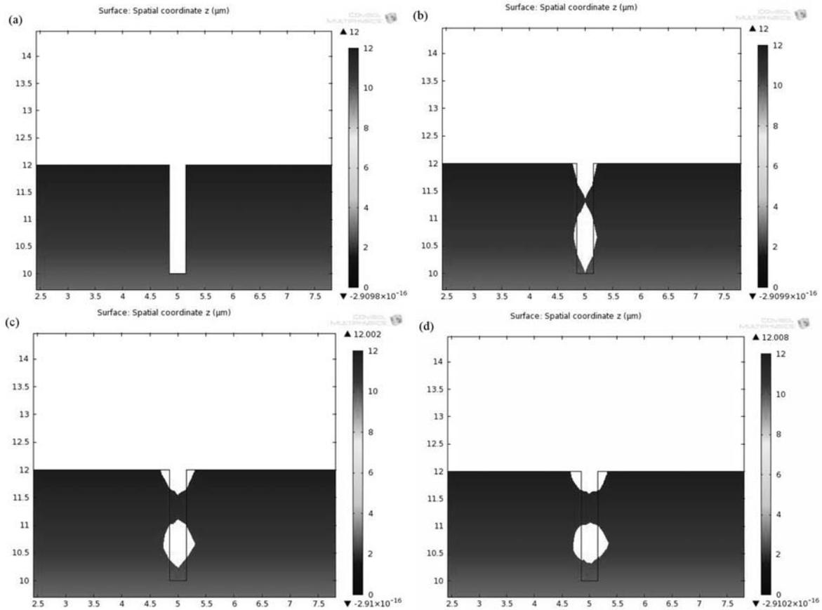
**Fig. 5** Shape evolution of a trench with a trench diameter of  $0.30\ \mu\text{m}$ , trench length of  $2\ \mu\text{m}$  at  $1100^\circ\text{C}$  after a) 0 s; b) 10 s; c) 20 s; d) 90 s.
