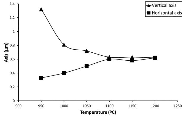
**Fig. 13** Diameters obtained after an annealing time of 70 s at different temperatures.
