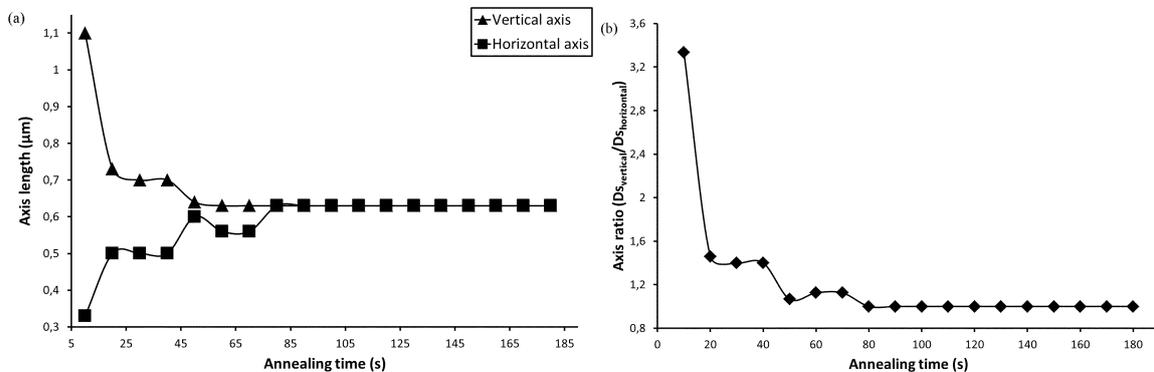
**Fig. 6** Ellipsoid (a) and axis ratio (b) evolution with the annealing time of a trench with a trench diameter of  $0.30\ \mu\text{m}$ , trench length of  $2\ \mu\text{m}$  at  $1100^\circ\text{C}$ .
