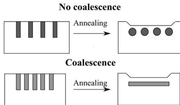
**Fig. 2** Scheme of the SON process with and without coalescence.
