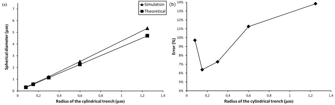
Fig. 7 Equilibrium spherical diameter depending on the cylindrical radius (a) and its relative error (b).
