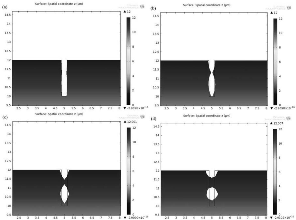
**Fig. 12** Geometry evolution after an annealing time of 70 s, geometrical parameters:  $L_c = 2 \mu\text{m}$  and cylindrical radius of  $0.15 \mu\text{m}$  at:  $900^\circ\text{C}$  (a);  $950^\circ\text{C}$  (b);  $1000^\circ\text{C}$ (c);  $1100^\circ\text{C}$  (d).
