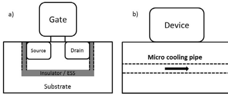
**Fig. 1** Basic scheme of two SON applications: a) SON transistor; b) micro cooling.
