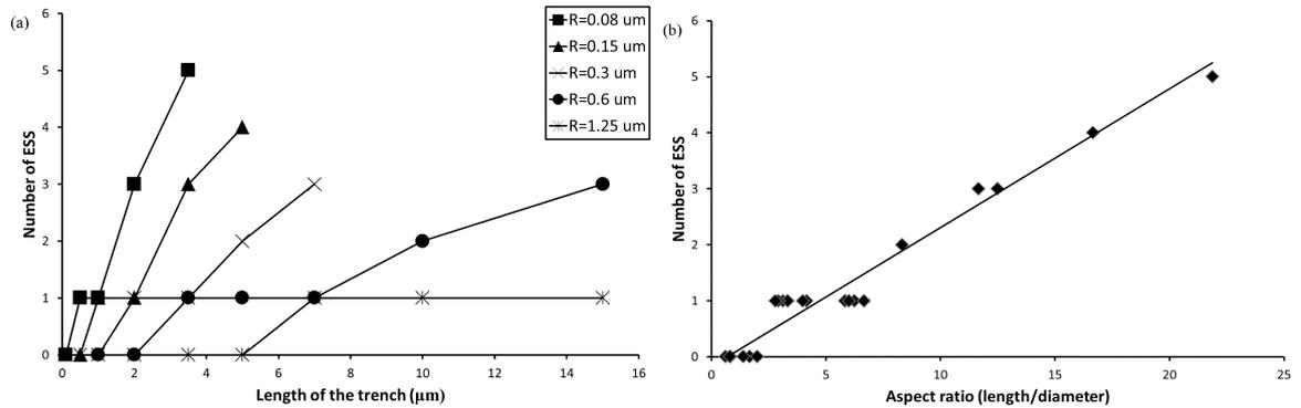
Fig. 8 Empty spaces in silicon (ESS) depending on the length of the trench (a) and on the aspect ratio (b).
