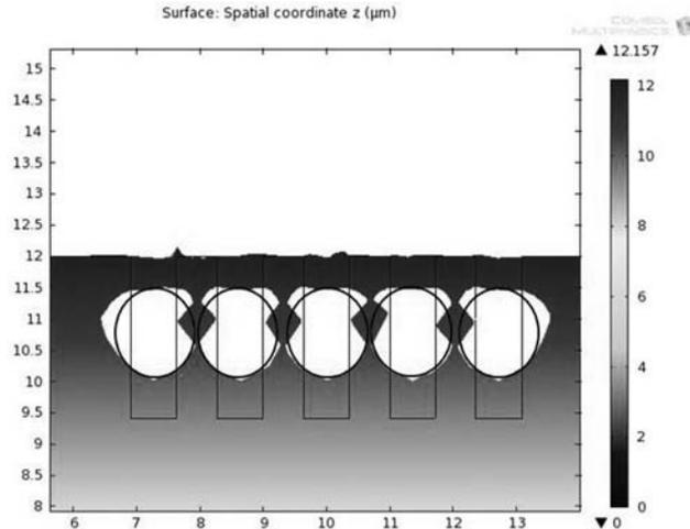
**Fig. 10** Simulation of the structure defined on [15]. Black ellipses represent the measured geometry; the relative error is 6.62% and 2.63% for vertical and horizontal axis, respectively.
