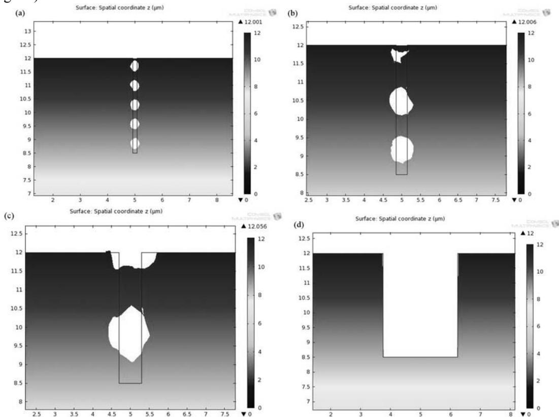
**Fig. 11** Geometry evolution after an annealing time of 1000s at 1100 °C,  $L_c = 3.5 \mu\text{m}$  and a cylindrical radius of 0.08  $\mu\text{m}$  (a); 0.15  $\mu\text{m}$  (b); 0.3  $\mu\text{m}$  (c); 1.25  $\mu\text{m}$  (d).
