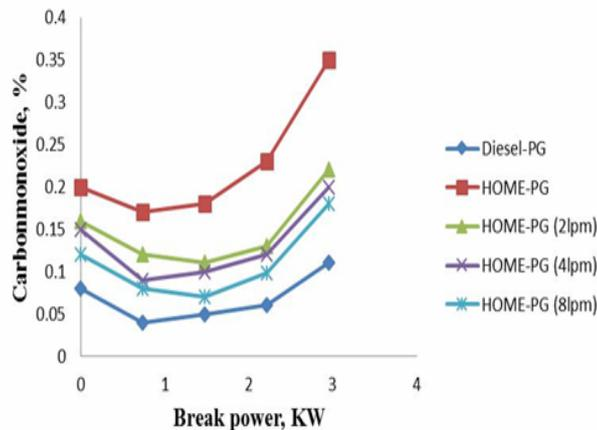
Fig. 10 Variation of carbon monoxide with brake power
