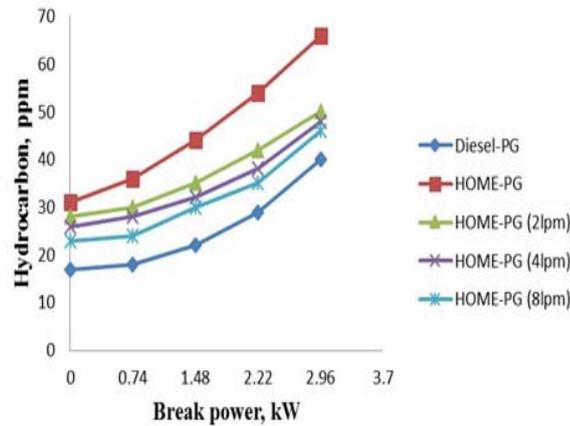
Fig. 9 Variation of hydrocarbon emission with brake power
