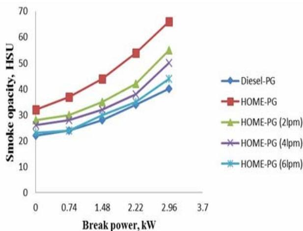
Fig. 8 Variation of smoke opacity with brake power
