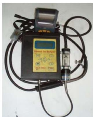
**Fig. 4** Exhaust gas analyser and Smoke-meter
