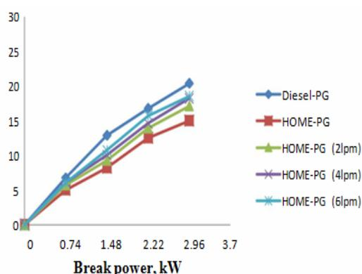
Fig. 7 Variation of brake thermal energy with brake power
