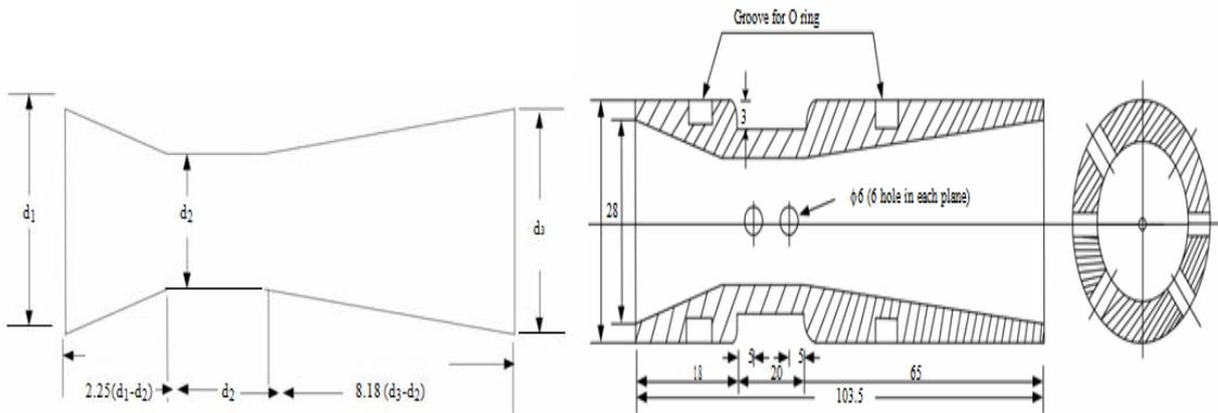
**Fig. 5** Dimensions of a standard venture
