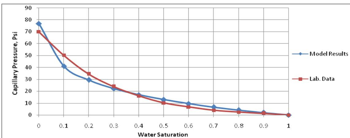
Fig. 8 Capillary pressure-saturation profile for well (HU-5)
