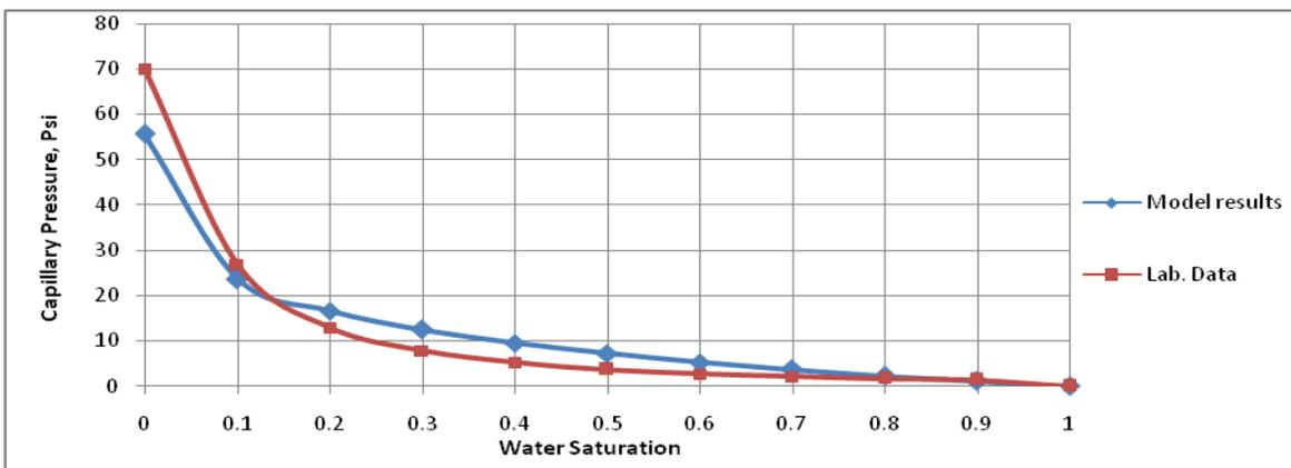
Fig. 6 Capillary pressure-saturation profile for well (HU-3)
