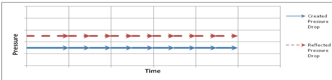
**Fig. 2** Schematic drawing shows the constant difference between the created and reflected pressure drops denoting the static capillary pressure across the fluid interface.
