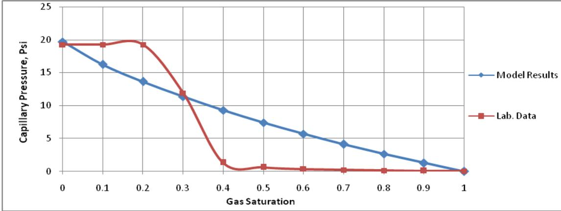
Fig. 10 Capillary pressure-saturation profile for well (HU-1)
