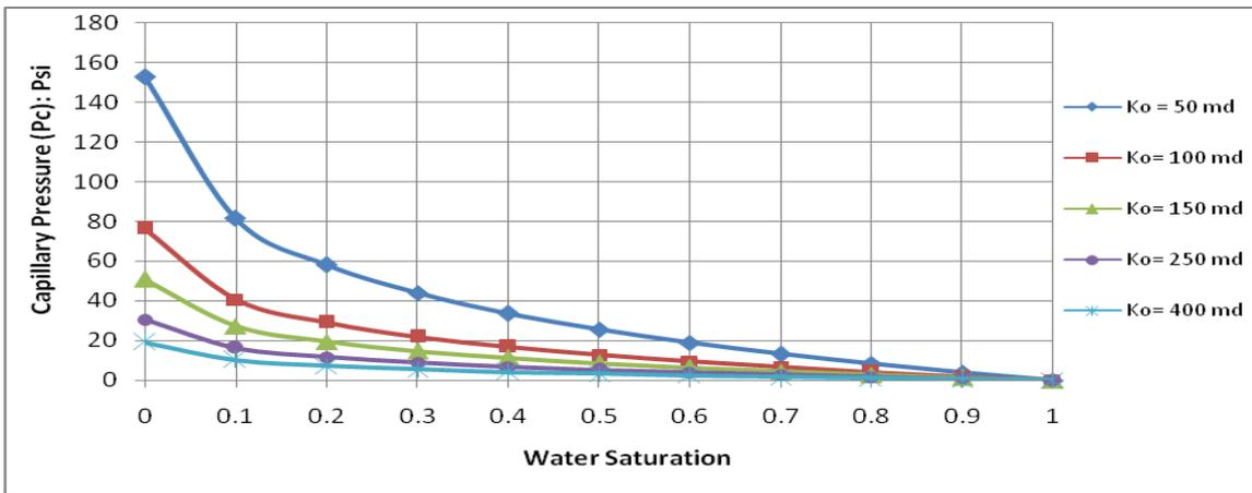
Fig. 14 Capillary pressure-saturation profiles generated by the presented model for different reservoir permeability values; taken  $Q_o = 500 \text{ STB/D}$ ,  $r_e=15000 \text{ ft}$ ,  $\mu_o = 2 \text{ cp}$ ,  $\mu_w=1 \text{ cp}$ ,  $\rho_w = 63.4 \text{ lb/ft}^3$ ,  $\rho_o = 53 \text{ lb/ft}^3$
