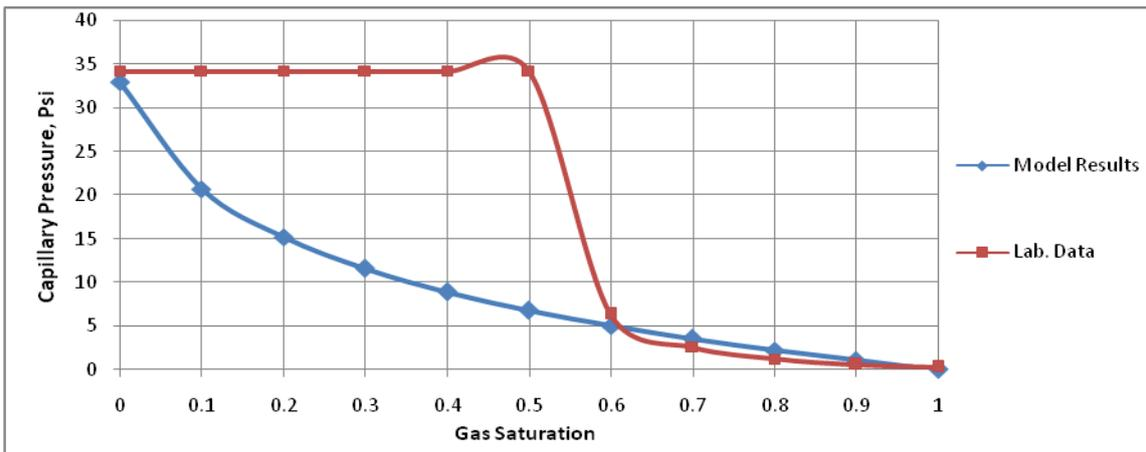
Fig. 12 Capillary pressure-saturation profile for well (HU-3)
