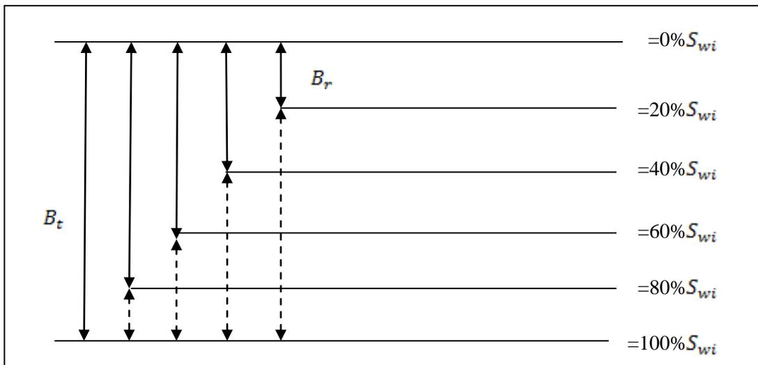
Fig. 3 Schematic drawing shows the change of total response function Reflecting the displacing fluid saturation
