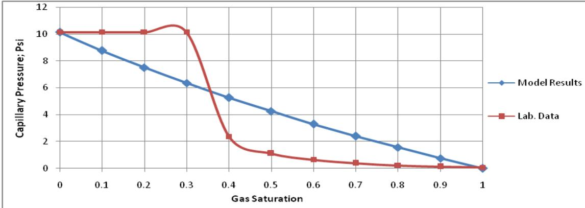
Fig. 13 Capillary pressure-saturation profile for well (HU-4)
