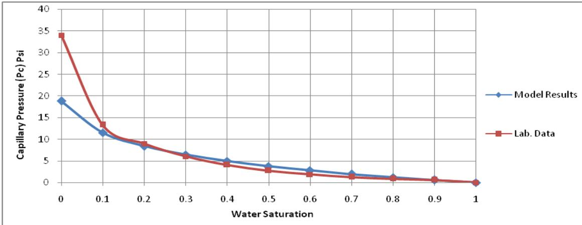
Fig. 5 Capillary pressure-saturation profile for well (HU-2)
