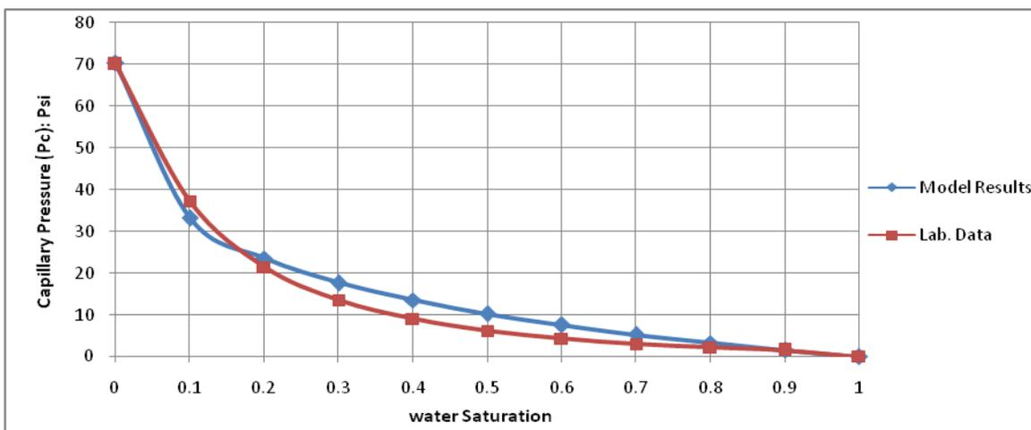
Fig. 7 Capillary pressure-saturation profile for well (HU-4)
