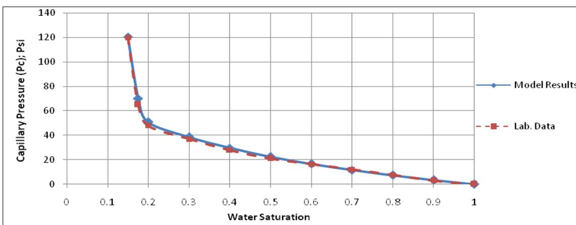
Fig. 9 Capillary pressure-saturation profile for well (HU-R1)
