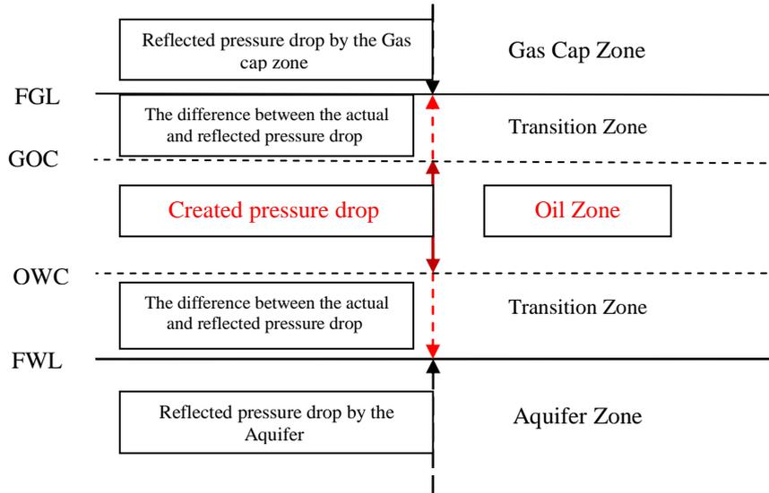
**Fig. 1** Schematic drawing for the created and reflected pressure drops at the fluid interface levels.
