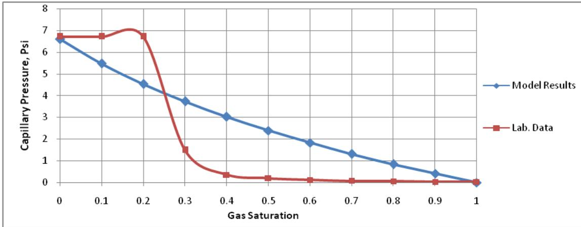
Fig. 11 Capillary pressure-saturation profile for well (HU-2)
