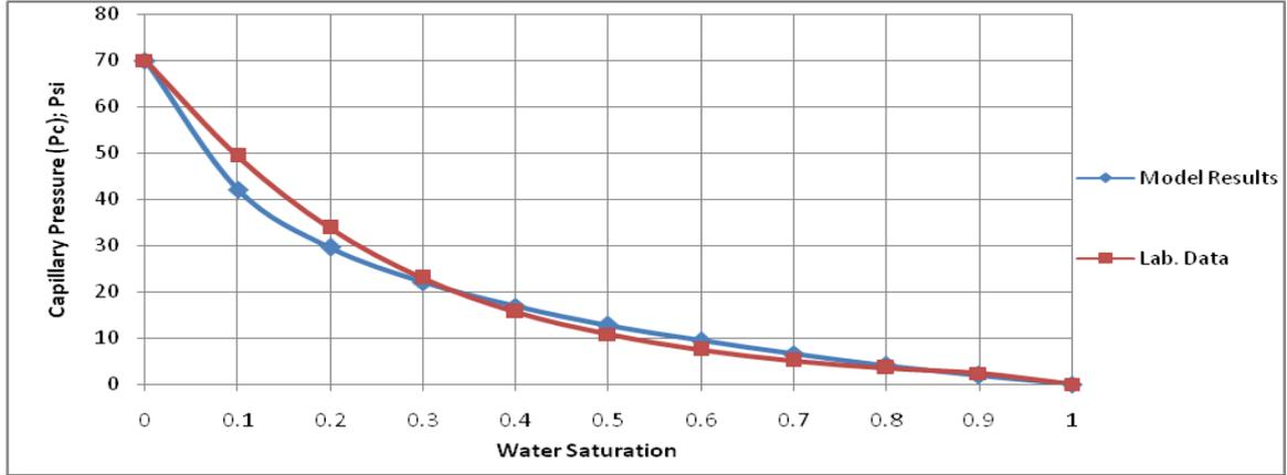
Fig. 4 Capillary pressure-saturation profile for well (HU-1)
