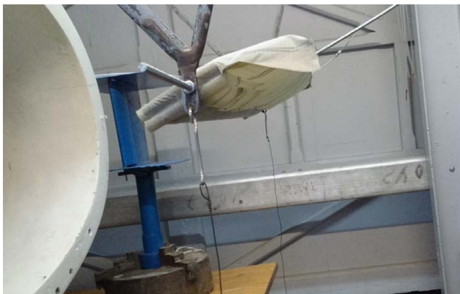
Fig. 10 Wing No: 4 – 30% rigid and 70% soft. Angle of attack is \alpha = 32^\circ
