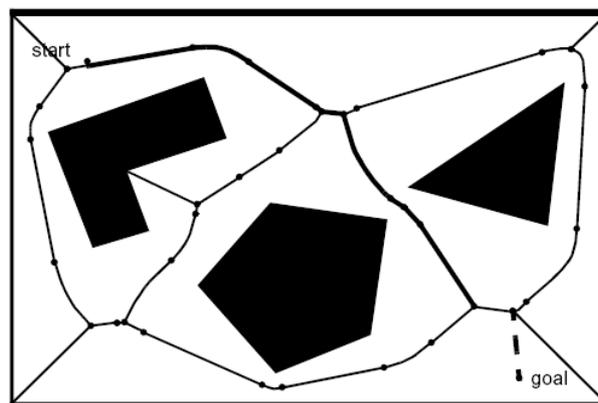
Fig 5 The Voronoi diagram for three polygon obstacles [2]
