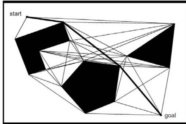
Fig 4 The Visibility graph for three polygon obstacles [2]
