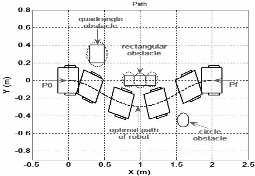
Fig 2 Multiple obstacle avoidance of the non-holonomic mobile manipulator [19]
