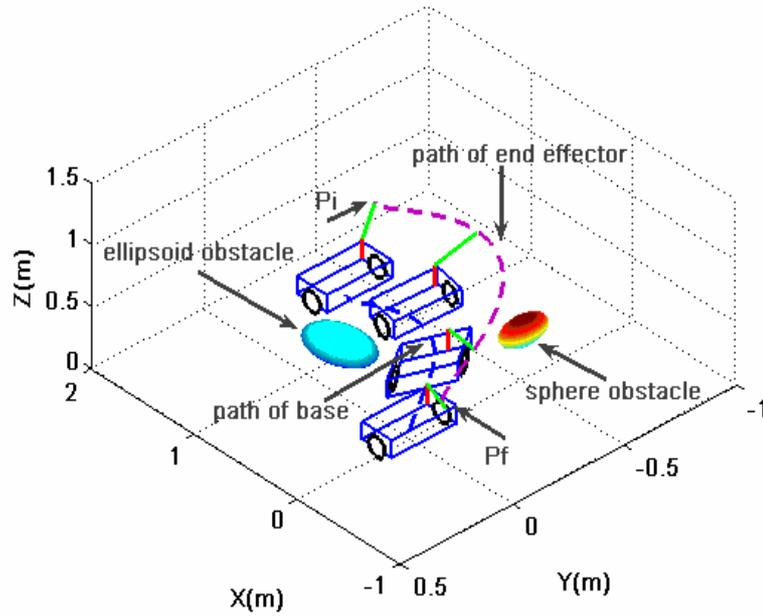
Fig 3 The Scout robot in the presence of spatial obstacles [20]
