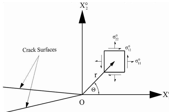
**Fig. 4** 2-D Coordinates near the crack tip.
