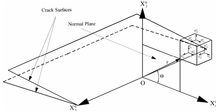
Fig. 5 3-D Coordinates near the crack tip.
