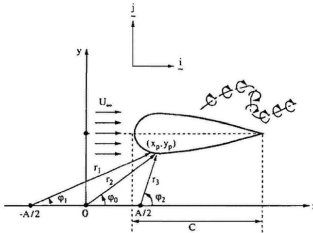
Fig. 2 Coordinate system for the 2D airfoil
