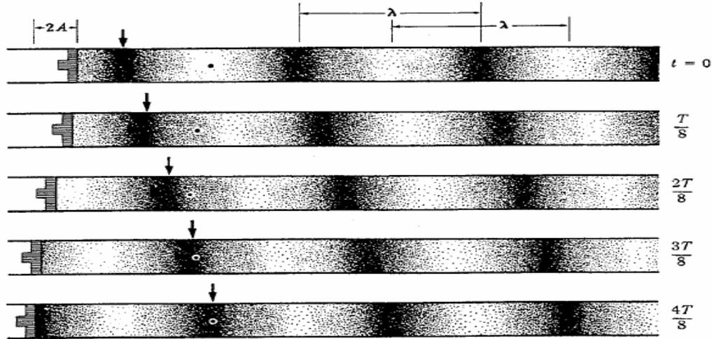
**Fig. 6** Sinusoidal longitudinal waves, traveling toward the right, at intervals 1/8 of a period. On the other hand, by differentiating the wave equation (5.1) results:
