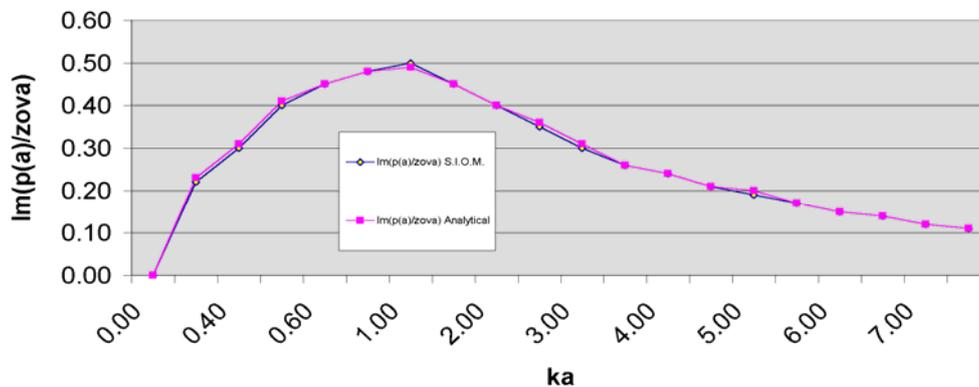
Fig. 3 Imaginary Part of Dimensionless Surface Acoustic Pressure of a Pulsating .
