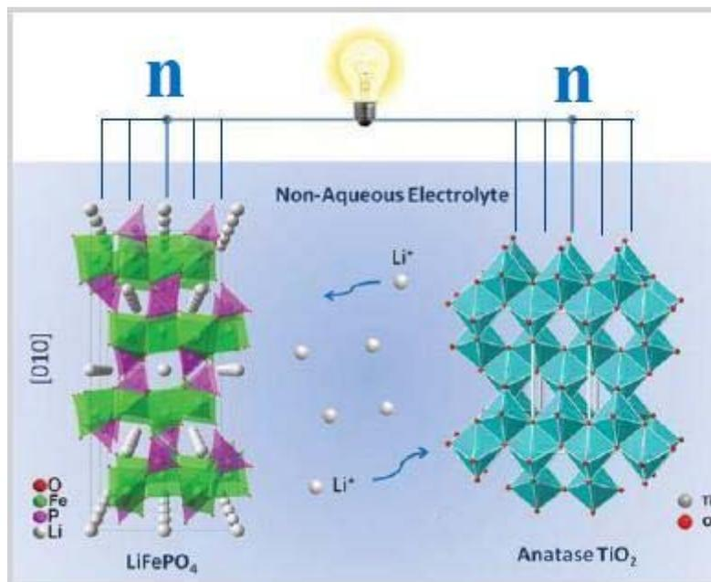
Fig. 1 A Lithium-Ion Battery with Intermediate Bands
