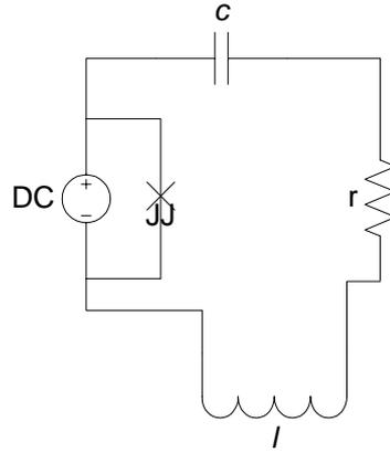
**Fig. 1** Josephson's generator connected in parallel to the RLC-circuit.
