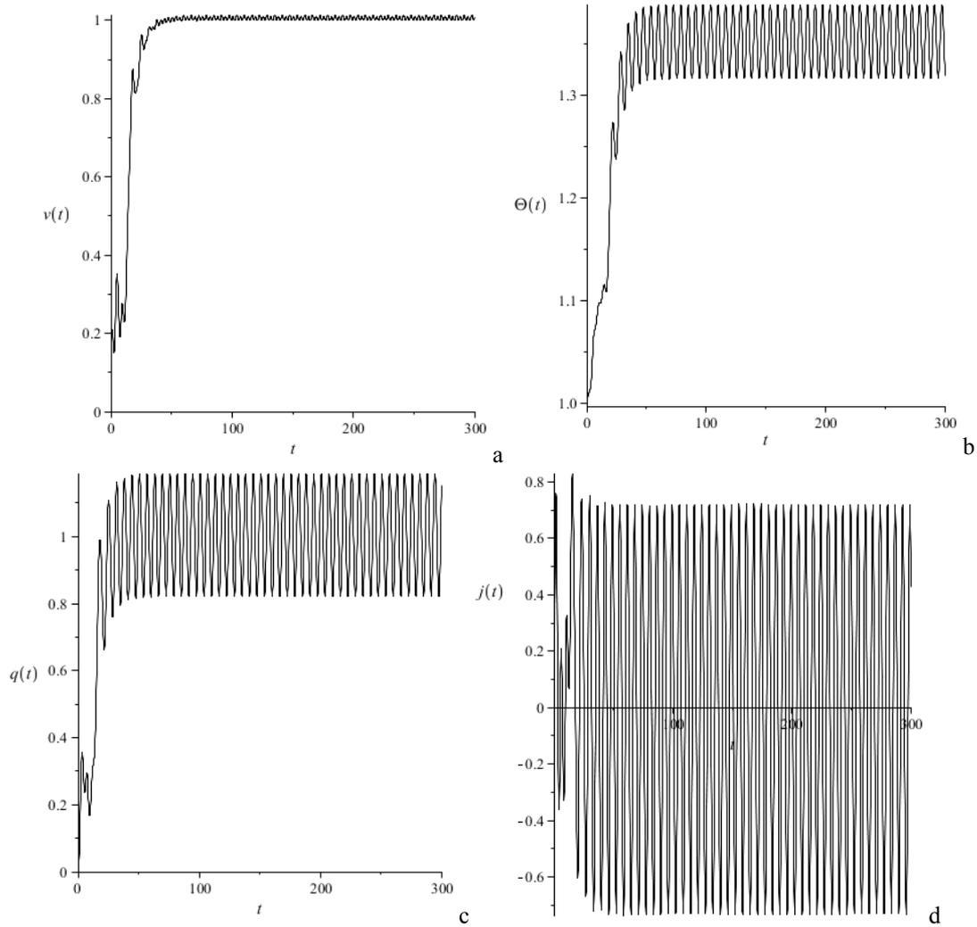
**Fig. 5** Dynamical response in the idle regime (a – voltage in the junction; b – temperature of the Josephson junction; c – charge in the RLC-circuit; d – current in the RLC-circuit).
