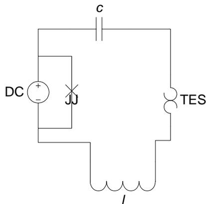
**Fig. 6** Self-excited resonant bolometer.
