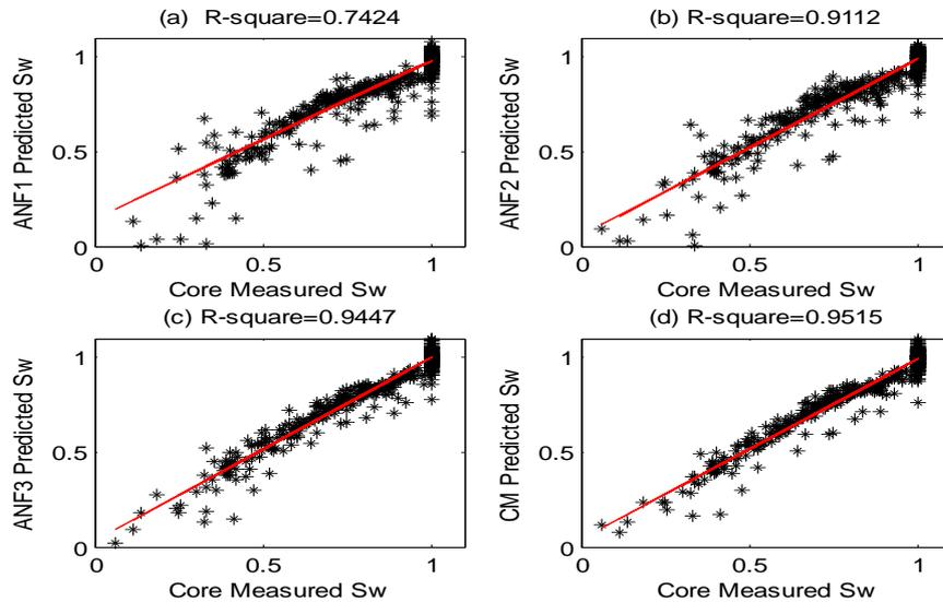
**Fig. 4** A scatter plot between core measured and a) ANF1, b) ANF2, c) ANF3, d) CM based on GA combined water saturation.
