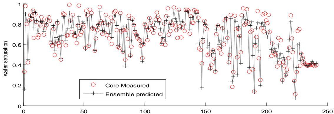
**Fig.5** Comparison of CM predicted and core measured water saturation versus depth.
