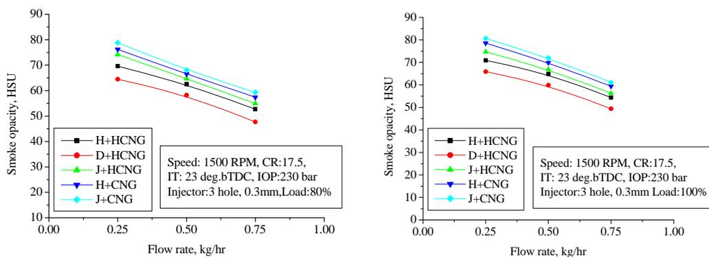
Fig. 3 Variation of Smoke opacity with flow rate
