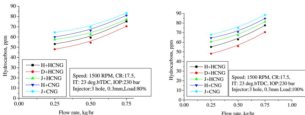
Fig. 4 Variation of HC with flow rate
