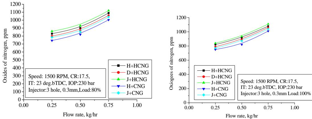
Fig. 6 Variation of NO<sub>x</sub> emission with flow rate
