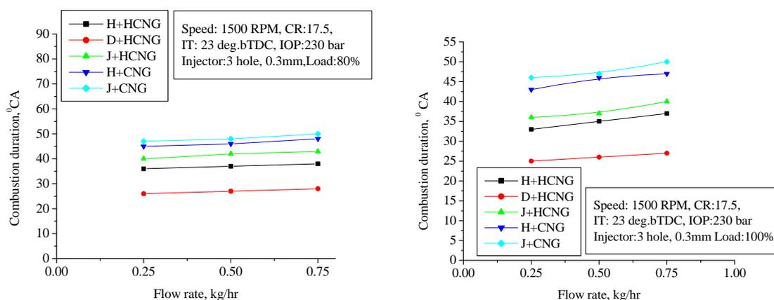
Fig. 8 Variation of combustion duration with flow rate
