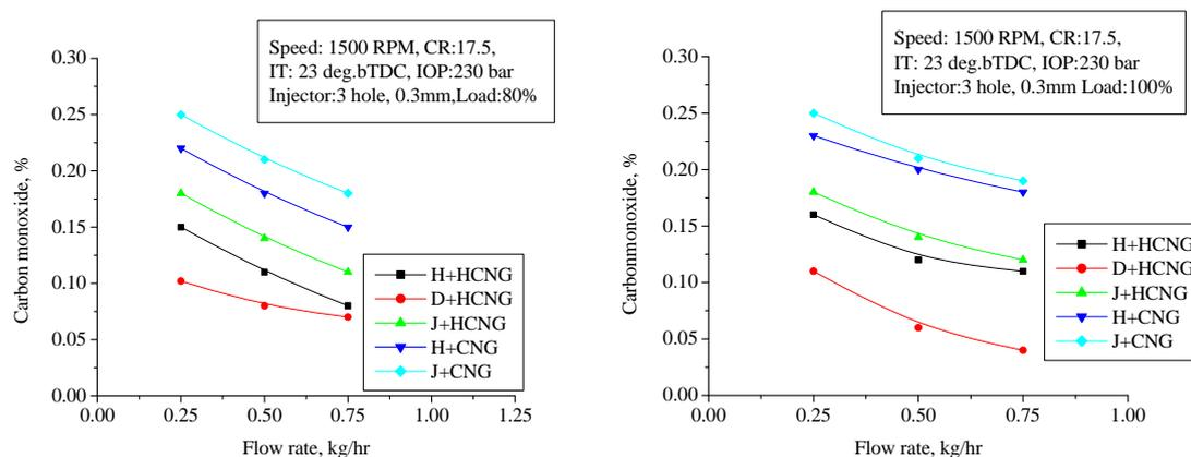
Fig. 5 Variation of CO with flow rate
