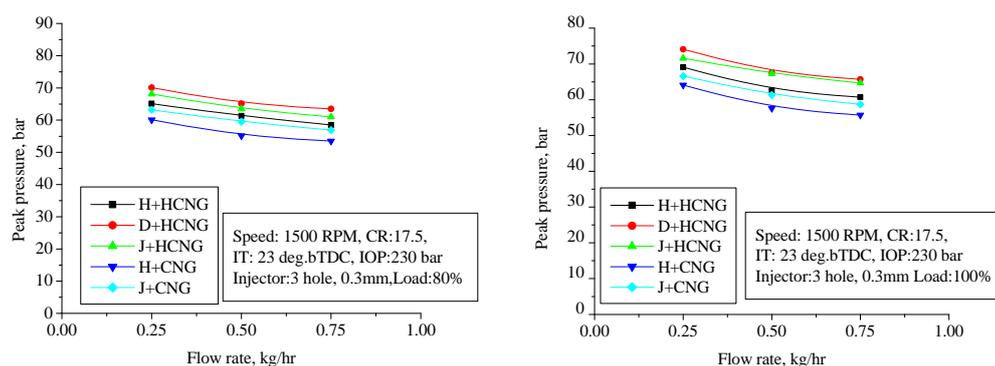
Fig. 9 Variation of peak pressure with flow rate
