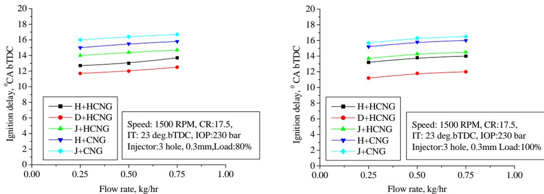
Fig. 7 Variation of ignition delay with flow rate
