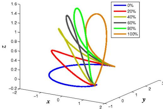
Fig. 2 Configurations rod according the load factor
