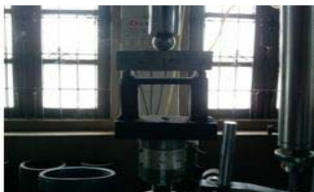
Fig. 1 Sample placements for three point load set-up
