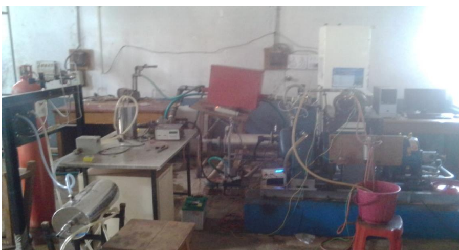
Fig. 4: Overall view of engine test rig with HCCI arrangement
