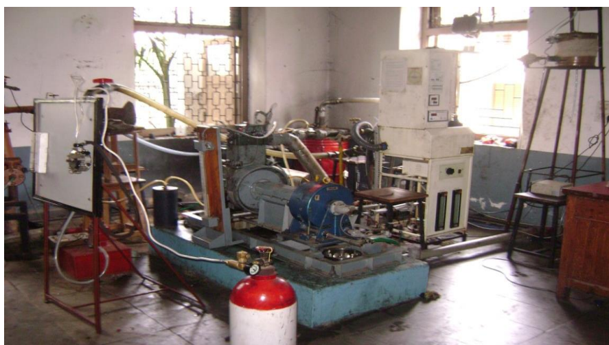
Fig.3 Overall view of engine test rig with dual fuel arrangement
